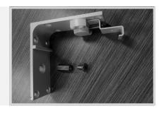
The screen box comes with 2 or 3 (depending on screen size) recessed cutouts for the L-shaped screen bracket to be installed, utilising the supplied Phillips type bolt and washer, which are screwed into the pre-fitted tee-nuts located in the roof of the screen box. We recommend that you also put at least 4 wood screws into the provided holes as a back-up measure against any bolt failure.
