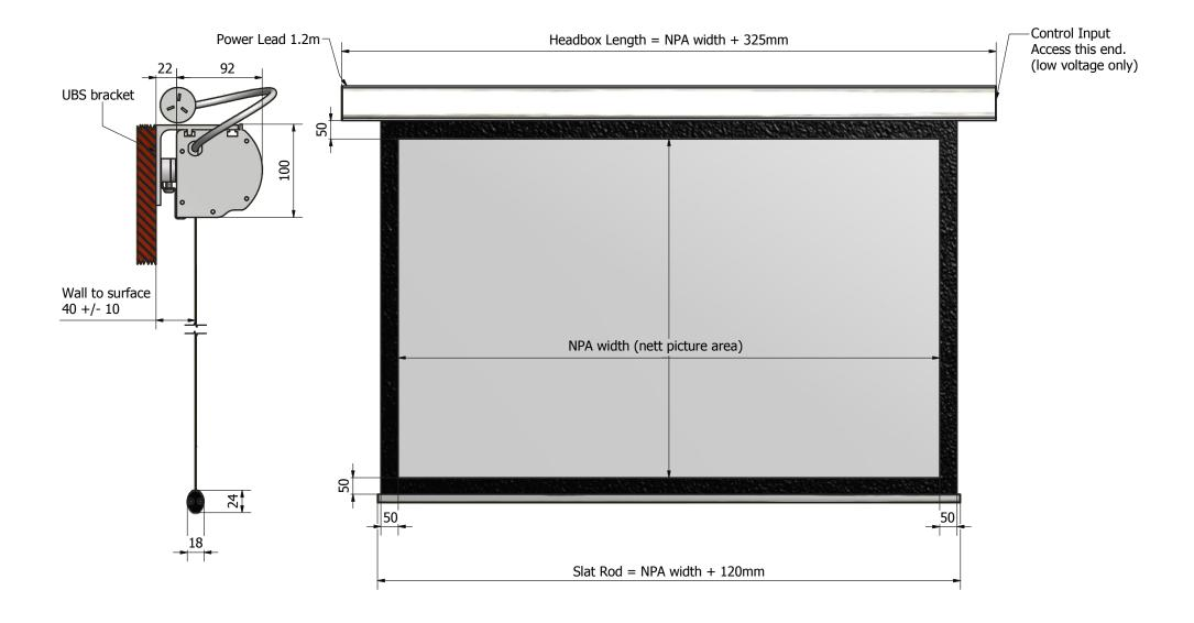
Manufacturing tolerance +/-5mm on headbox and slatrod All dimensions are in (mm) If installed in ceiling always allow for removal for servicing.
