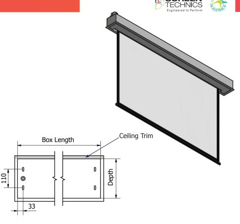
4 off Captive Nut Positions Ø5/16 Whitworth 2 at either end
