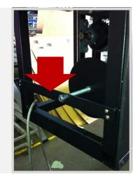
STEP 4. Screw on left- and right-hand timber covers.
