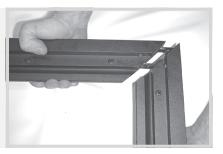
STEP 3. Push the two corners of the frame together. You may need to use a plastic or wooden mallet (not metal) to achieve this result, please use mallet very softly so not to damage finish, although a good wiggle of the frame will normally suffice.
