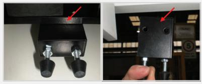
STEP 4. Remove rubber block on the right hand side only using a 4mm Allen key
