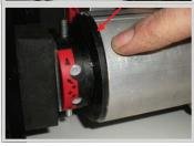
STEP 8. Replace rubber block using a 4mm Allen Key
