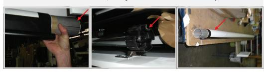
STEP 6. Slide the replacement screen surface and tube over the motor, making sure that the tape on the motor drive lines up with the key way in the screen surface tube. (Shown in pictures below)
