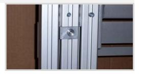
STEP 3. Run the mechanism all the way down (panel should be removed at this stage) and look for the white nylon bearing at the top of the outside groove, the spacer is fitted hard up underneath this spacer, using the Allen key bolt supplied.
