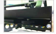
STEP 2. Removal of the plate for drilling and fitting is achieved by undoing the 2 off Allen key bolts along the front underside edge of the mounting plate, and pulling the plate forward.
