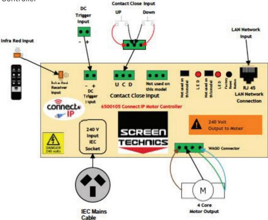
All inputs on module 1 are accessed by removing right hand end cap of screen canister
