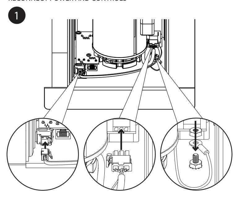
Plug in the motor control, power, and grounding wires making sure all cables are routed away from the moving tube.
