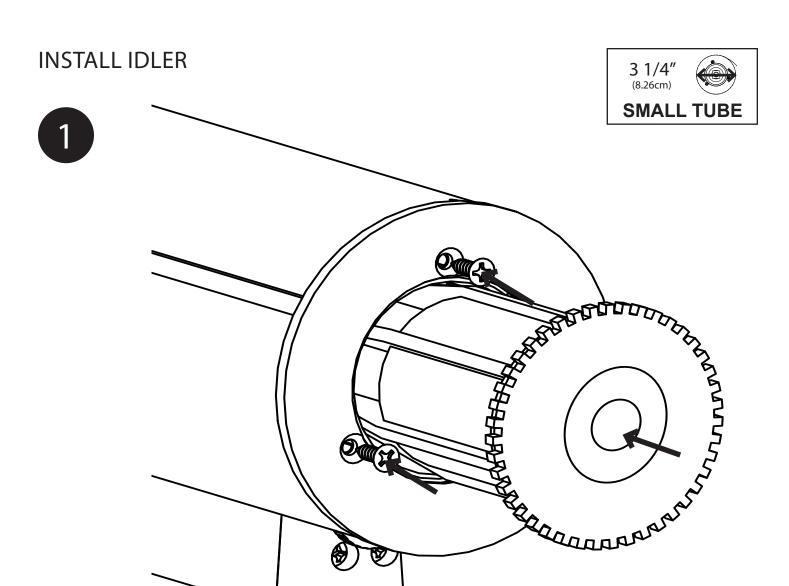
Slide the idler into the opposite end of the tube and secure with 3 phillips head screws. Make sure the idler is retracted all the way in preparation for installation into the case. Turn to page 18 to install the screen in the case.
