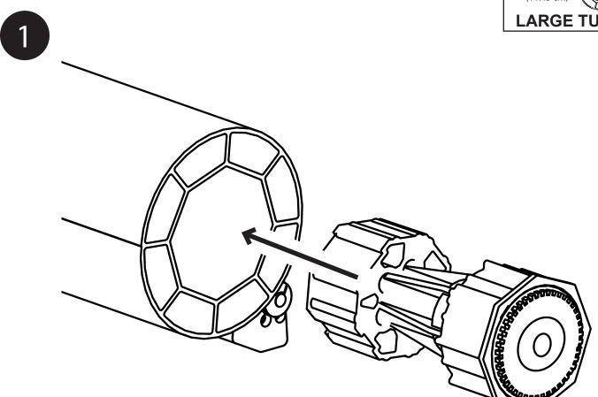
Slide the idler assembly into the opposite end of the tube.
