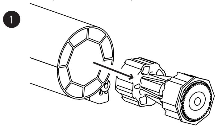
Pull the idler assembly completely out of the tube.
