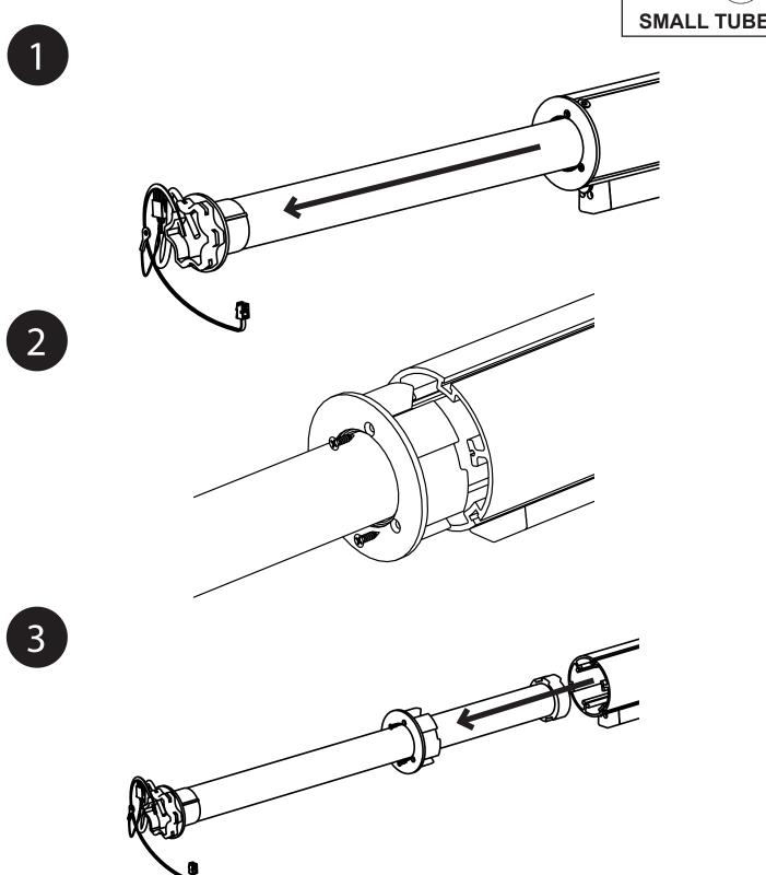
Slide the motor out to get access to the retaining screws. Remove and set aside the retaining screws, then completely remove the motor.
