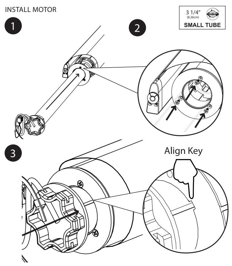
Slide the motor partially into the tube and secure the black plastic piece on the motor to the tube with the phillips head screws. Then push the motor all the way into the tube making sure to align the key on the motor with the key in black piece scured to the tube.
