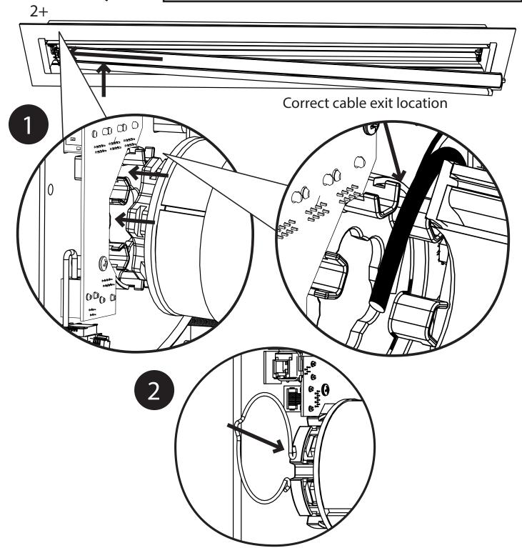
Push the motor into the motor bracket at the left end of the case taking care to make sure the motor power and control cables do not become pinched and exit at about 1 o-clock as shown. Then install the motor retaining ring.
