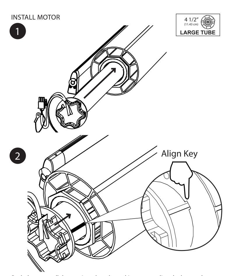
Push the motor all the way into the tube making sure to align the key on the motor with the key in black piece inserted into the tube.
