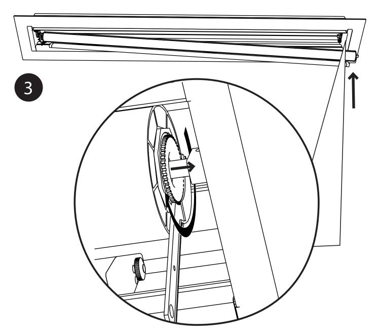
Raise the right end up and align the idler shaft with the bushing on the right side of the case, then turn the teeth on the idler clockwise to extend the idler shaft into the bushing hole. Keep turning until the you feel the teeth stop.
