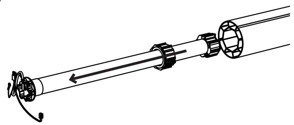
Pull the motor assembly completely out of the tube.
