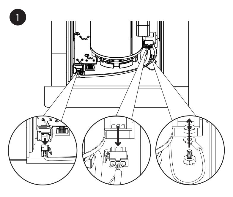
Disconnect the control, power, and grounding cables from the left side of the case.
