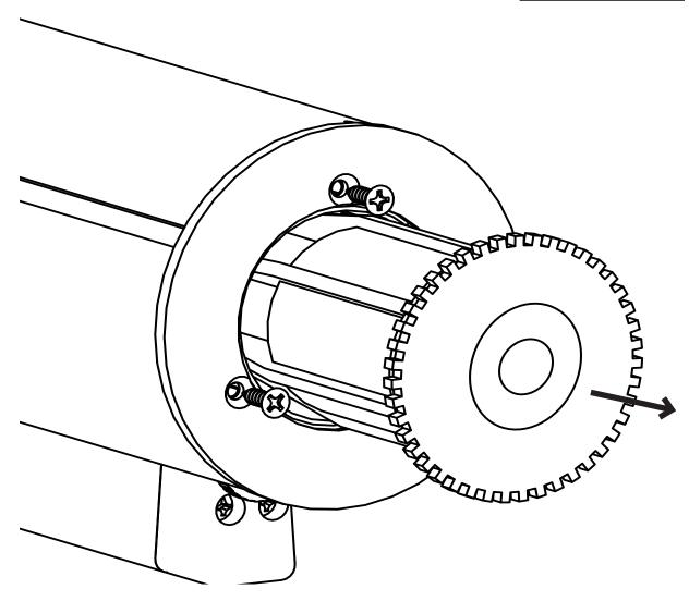
Pull the idler assembly out to access the screws, then remove the screws, and finally remove the idler assembly.
