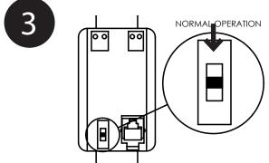
Slide the switch on the back to the upper position. Then hold the up button to raise screen up into the case as shown. When the screen is in the correct position then slide the switch down to the normal operating position.
