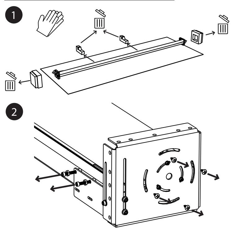
Open the fanfold box and discard the foam. Then remove the straps and screws from the wieght bar cradles. Then remove the screws from the shipping end plates.
