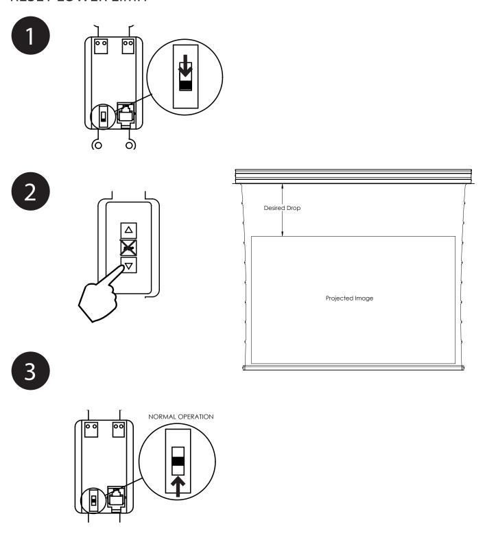
Plug in the wall switch to any port on the control board, slide the switch on the back to the lower position. Then hold the down button to lower the screen to the desired drop. Once the screen is open to the desired position then slide the switch up to the normal operating position.
