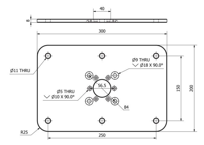
Manufacturing tolerance +/- 5mm All dimensions are in (mm) If installed in ceiling always allow for removal for servicing.
