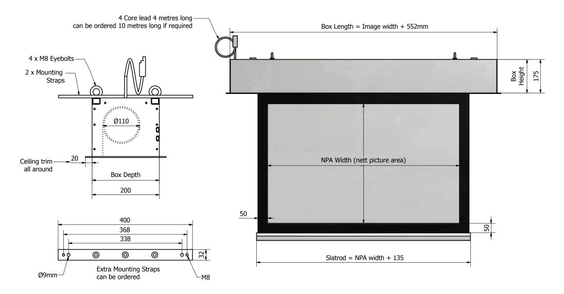
Manufacturing tolerance +/- 5mm on in ceiling box and slatrod All dimensions are in (mm) Always allow for removal of screen for servicing.
