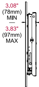
SIDE VIEW COLLAPSED
